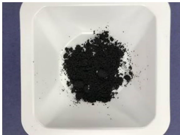
Figure 3: CMTT particles after cryogenic milling.
