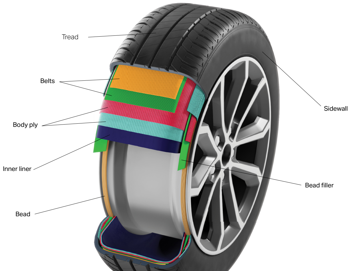
Figure 5: Tire structure - A representation of the structural composition of a typical passenger vehicle or light truck tire. The structural composition of tires differs according to tire type and tire application.
